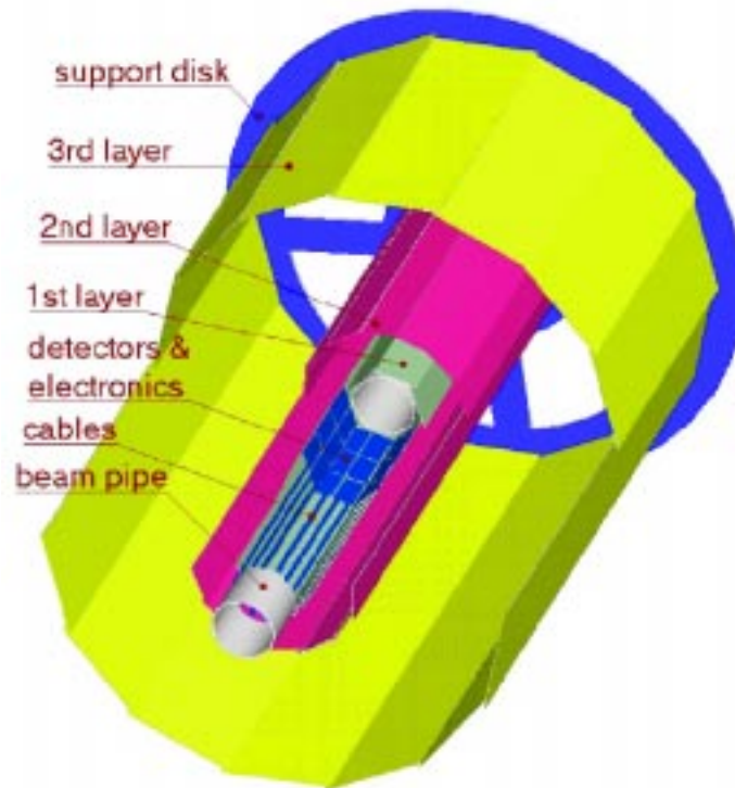
Figure 2.1.2: General layout of the barrel section of the hybrid pixel-based vertex detector.
