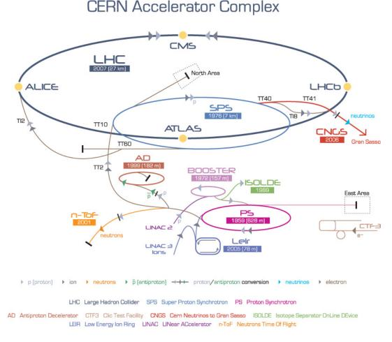
**Figure 1:** The CERN accelerator complex
