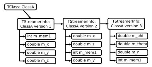
Figure 17: The TStreamernfo objects associated with TClass for a sample hierarchy
