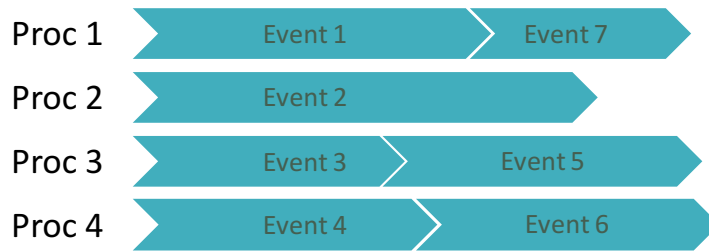
Figure 33: Processing model of AthenaMP. The flow does not change with respect to Athena except that all processes pick events from a single queue, balancing the load between processes.
