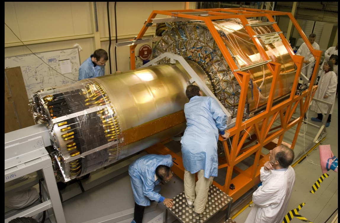
example: ATLAS TRT measured before and after insertion of the SCT
